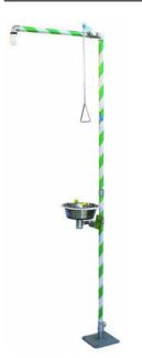
Size Emergency and eye shower MBS150-30 stainless steel (1¼") Article number 999999979 Material Stainless steel bath, Stainless steel pipes, Plastic shower head RVS Pipework Operation Stainless steel push bar and stainless steel pull bar Water flow Shower 80 ltr/min, bath 12 ltr/min. 1<sup>1</sup>/<sub>4</sub>" BSP internal thread Water supply
